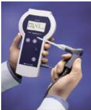
Figure 3. Sublingual capnometry measures sublingual PCO 2 , which correlates with a gastric intracellular pH.
